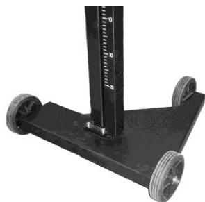
The optical chamber is adjustable in height by means of slides on precise, silent, plastic runners, balanced by a spring, mounted inside of a laminate cover, where a centimeter scale is indicated for exact positioning with respect to the headlight.
