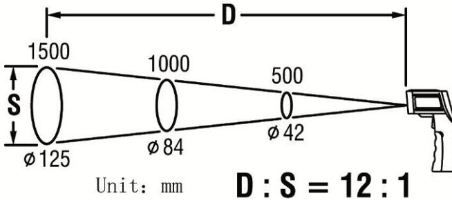
i.e. at a distance of 100 cm, the measurement area is approx. 8.5 cm in size.
